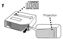
Make sure the disc magazine is the right way up with the "disc" logo on the top.Pull the tray out by the projection.
