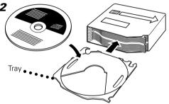
Place the disc on the tray with the label facing upwards. Insert the tray into the disc magazine until it locks. Check that the discs and trays are inserted properly. The discs are numbered from the bottom from 1 to 6 or 10.
